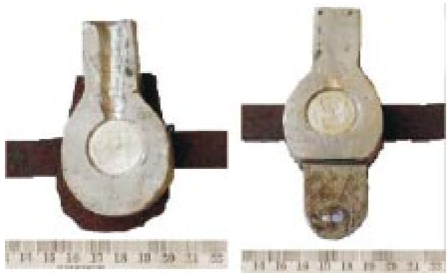
Figure 3: The Dies used for making the coins.
