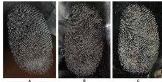
Figure 6. Fingerprint developed on Aluminium foil using Rice flour. Note: A – 0h; B- 6h; C- 72h.
