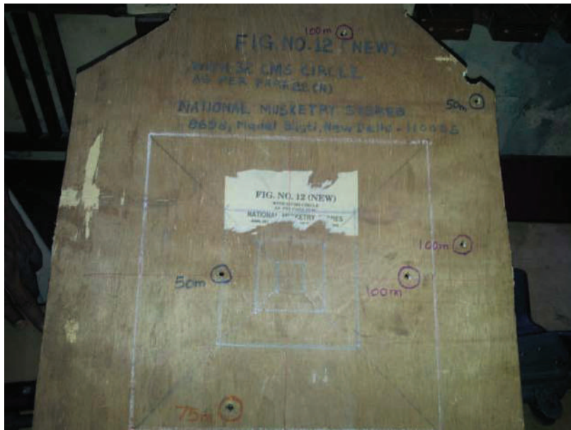
Figure showing penetration of rubber/plastic bullet fired from
