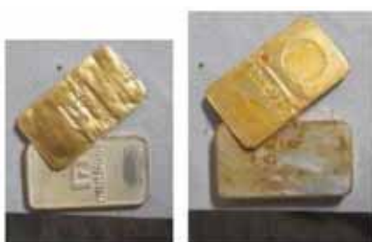
Fig. 5: The inner portion of golden bullions after removing the gold sheet
