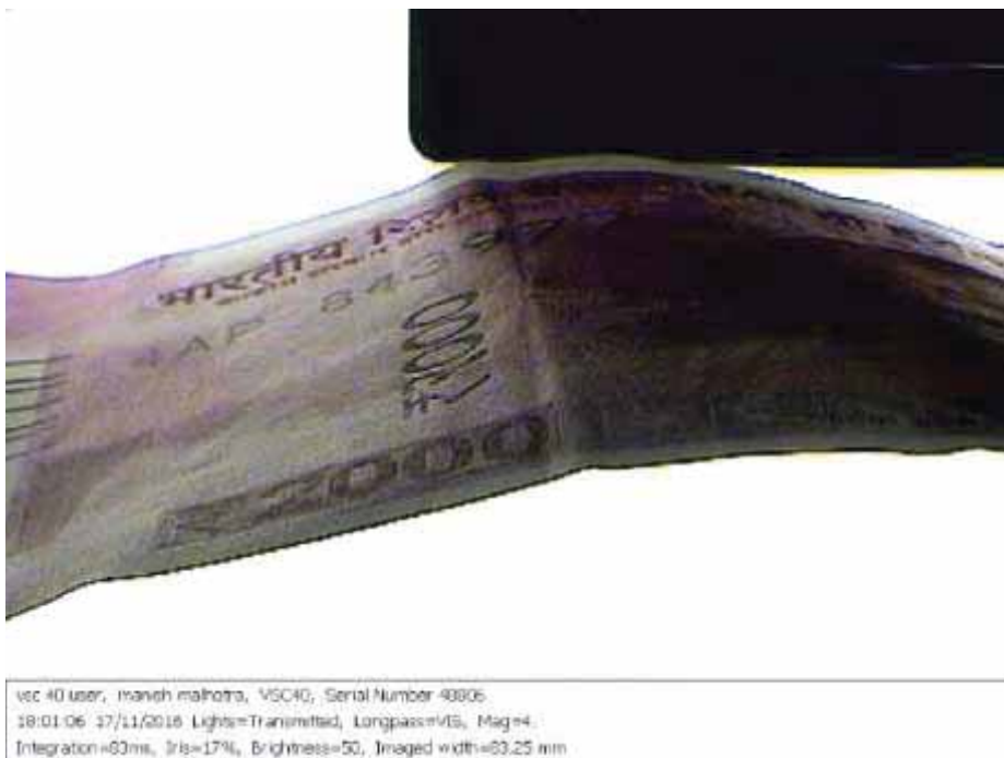
Figure 3: Latent image (Light: Transmitted, Longpass: VIS, Mag:4) in ₹2000 note
