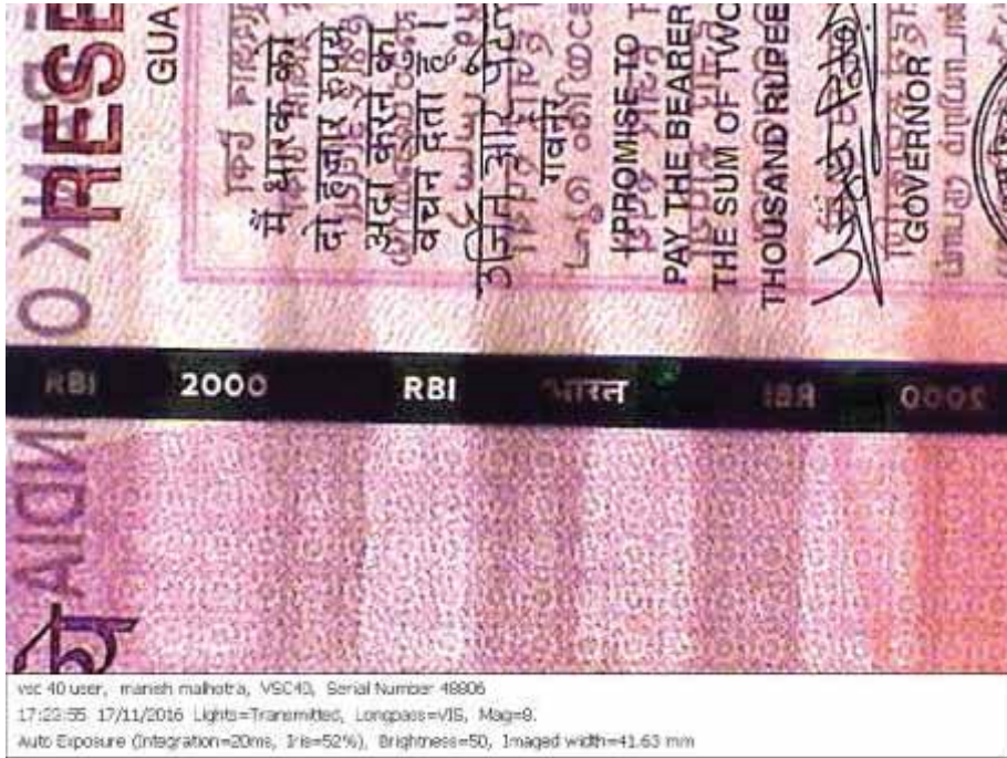
Figure 13: Optical variable ink (Light: OVD Viewer, Longpass: OFF, Mag:2.26) in ₹2000 note
