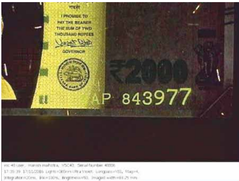
Figure 11: Watermarks (Light: Transmitted, Longpass: VIS, Mag:2.26) in ₹2000 note
