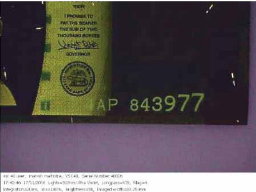
Figure 9: Serial number (Light: UV 312, Longpass: VIS, Mag:4) in ₹2000 note
