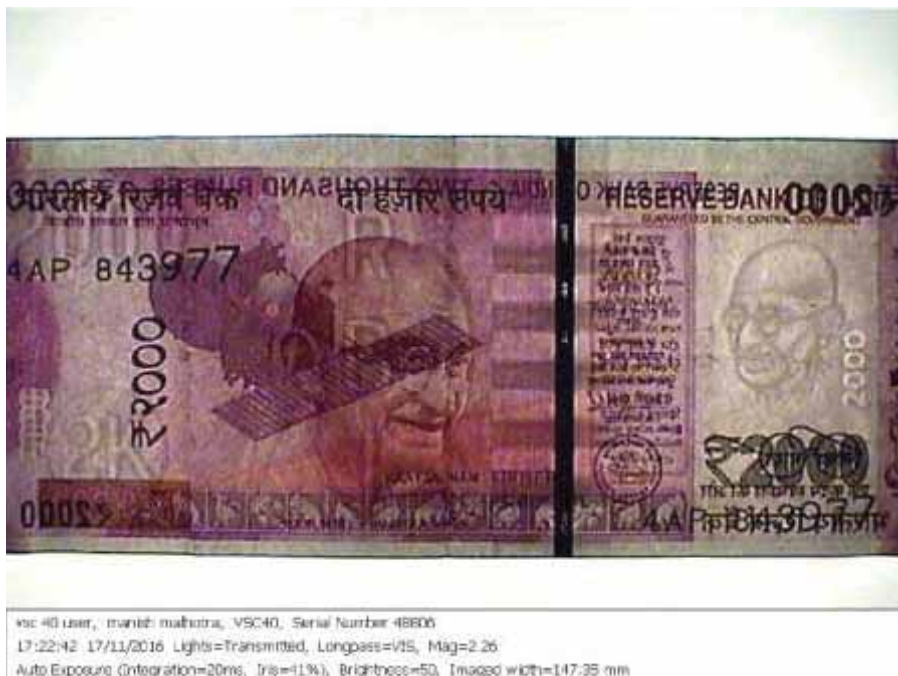
Figure 11: Watermarks (Light: Transmitted, Longpass: VIS, Mag:2.26) in ₹2000 note
