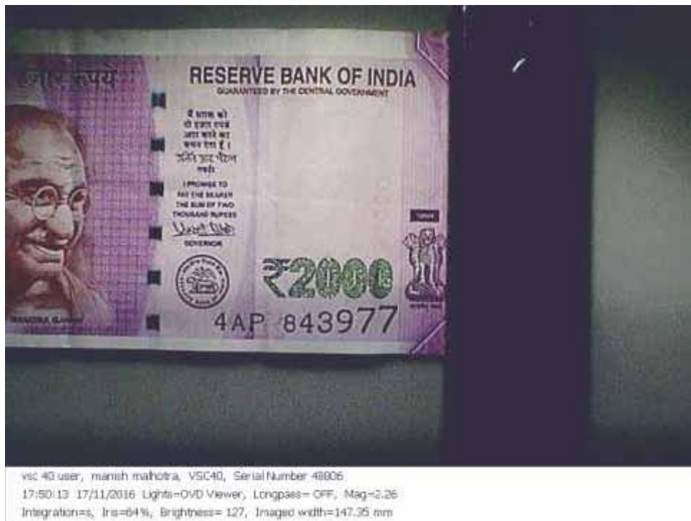
Figure 14: Optical variable ink (Light: OVD Viewer, Longpass: OFF, Mag:2.26) in ₹2000 note
