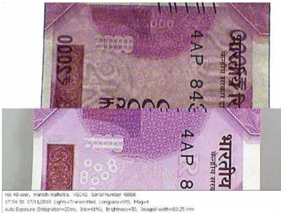
Figure 7: Fluorescent image (Light: UV 365, Longpass: VIS, Mag:2.26) in ₹2000 note
