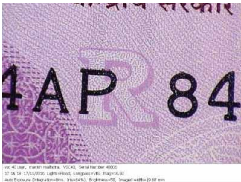
Figure 1: Micro lettering (Light: Flood, Longpass: VIS, Mag: 16.92) in ₹2000 note
