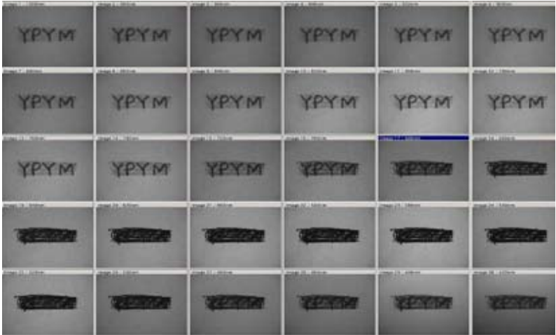
Fig.4. Hyperspectral images of Exhibit (a) (where pencil writing obliterated with ball pen) at 30 different wavelengths ranges from 400nm to 1000nm with a step of 20nm.
